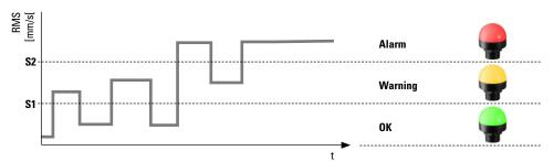
The transition points S1 and S2 between the warning levels can be individually parameterized as switching outputs in the vibration sensor.
