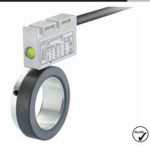
Thanks to its installation depth of only 16 mm, the bearingless magnetic rotary encoder RLI50, comprising a magnetic ring and sensor head, is ideally suited for plants and machinery where space is very tight. The non-contact measuring principle allows for error-free use even under harsh environmental conditions, as well as ensuring a long service life. In contrast to our measuring system RLI20, a single reference signal is also implemented here.
